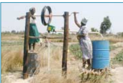
Using the rope pump
