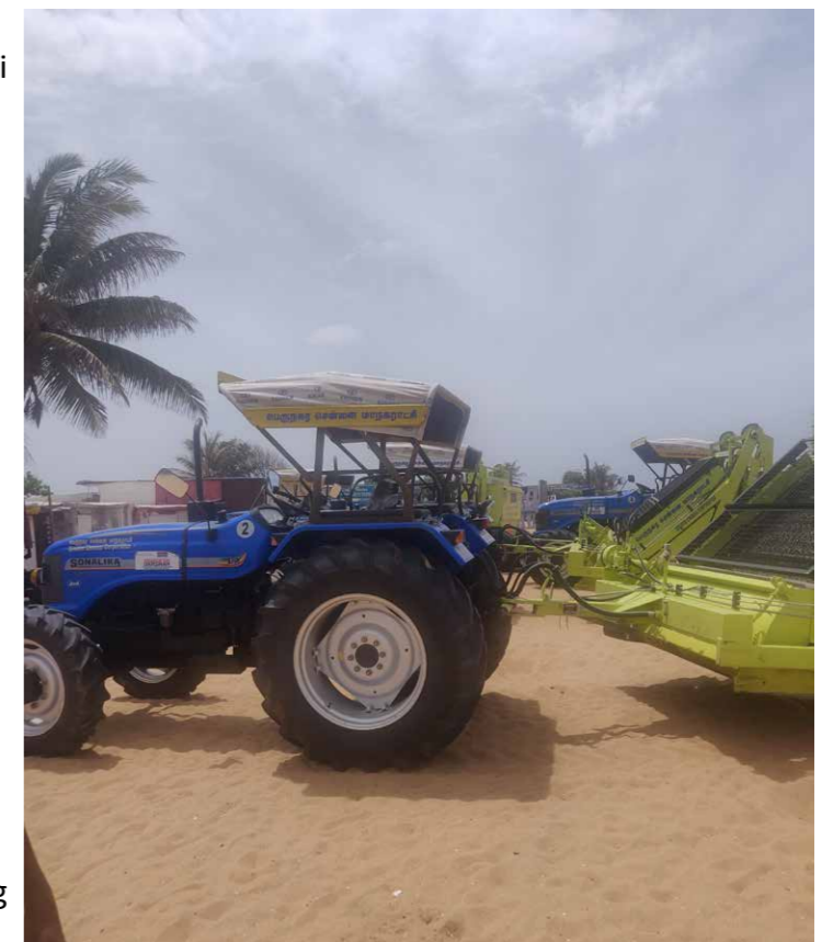
Figure 15: Tractor-driven beach cleaning machines for cleaning plastic waste from Marina beach, Tamil Nadu (July 2019)
